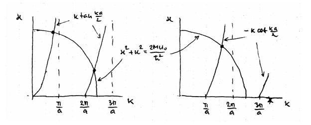
On figures we see that inside the well there is always finite number of possible energy states (minimum is 1 state) and it depends how large  $U_0$  is. In our case thare is three energy levels.
