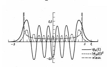
n = 10. The classical and quantum oscillators behave differently, but in the case of large n we see that the average of quantum probability distribution is practically equal to the probability of classical oscillator. That is the general result, since in the limit of large quantum numbers we have the same results as in classical physics.
